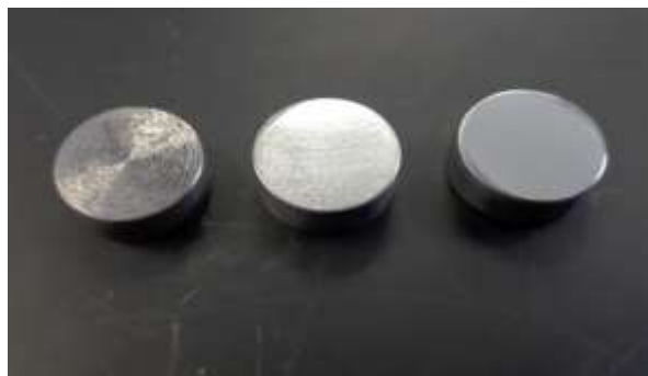
Figure 1. AISI 1018 steel samples before and after grinding/polishing
